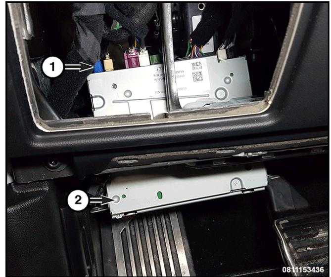
3. Working inside the storage compartment, install the ETM (2) on the instrument panel carrier frame.
