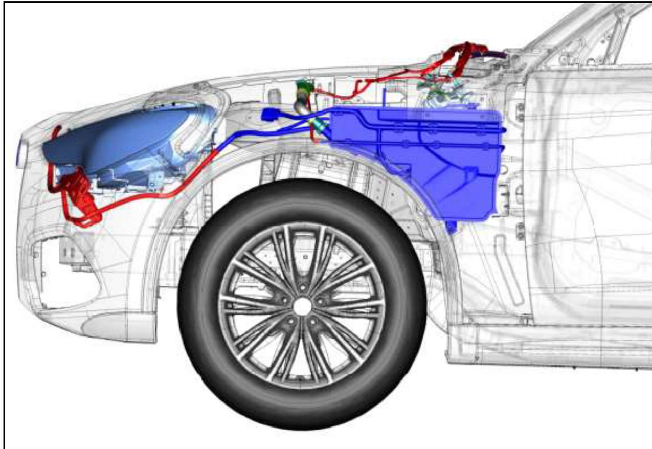
The system consists of a reservoir for the washer fluid, front nozzles inserted directly on the windshield wiper blades, connecting hoses and a sprayer nozzle in the tailgate spoiler.
