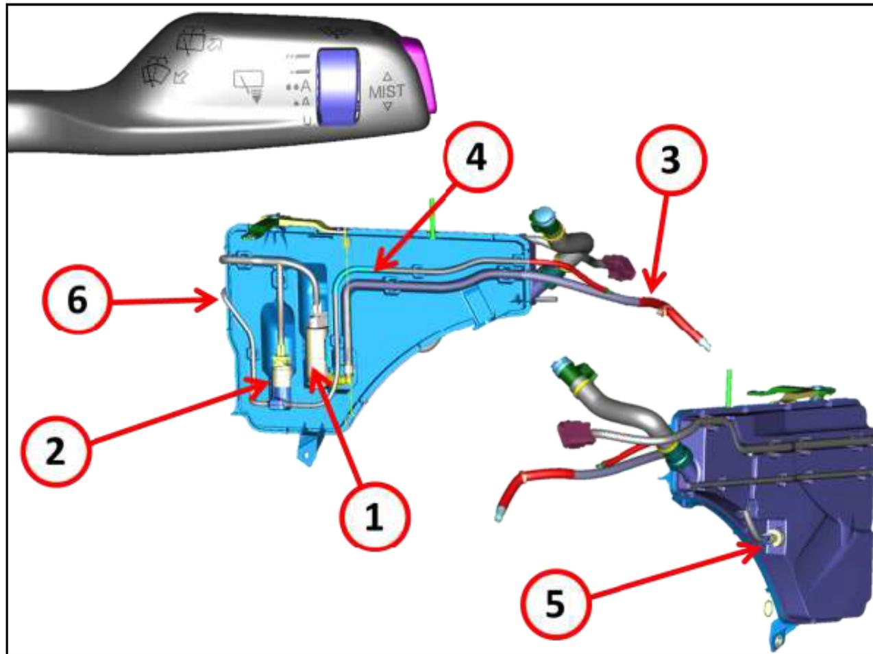
The BCM sends current to the windshield washer system pump when the right stalk is pulled towards the driver for the windshield wiper or pushed for the rear window wiper.
