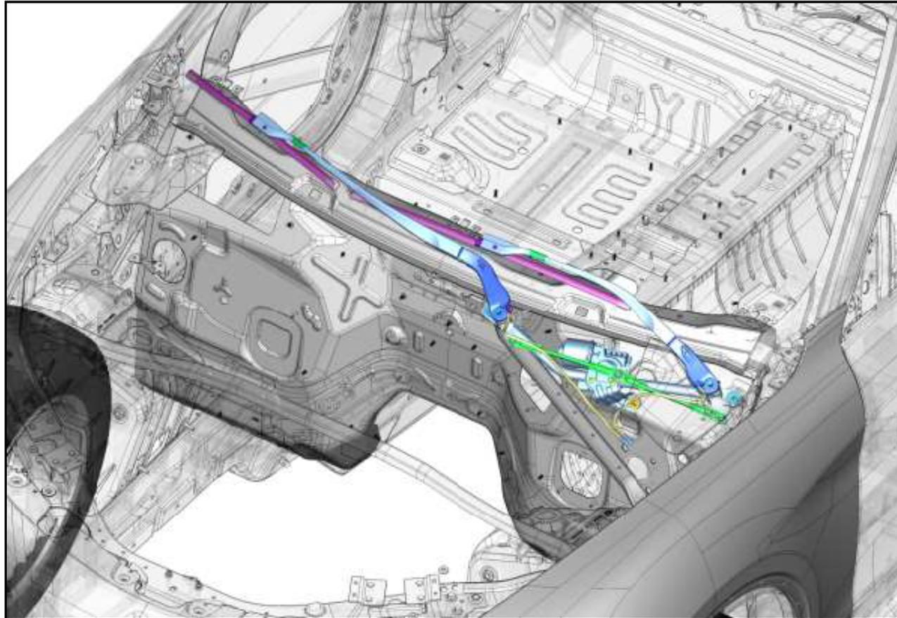
The windshield wiper mechanism is located behind the cowl trim, just below the windshield.
