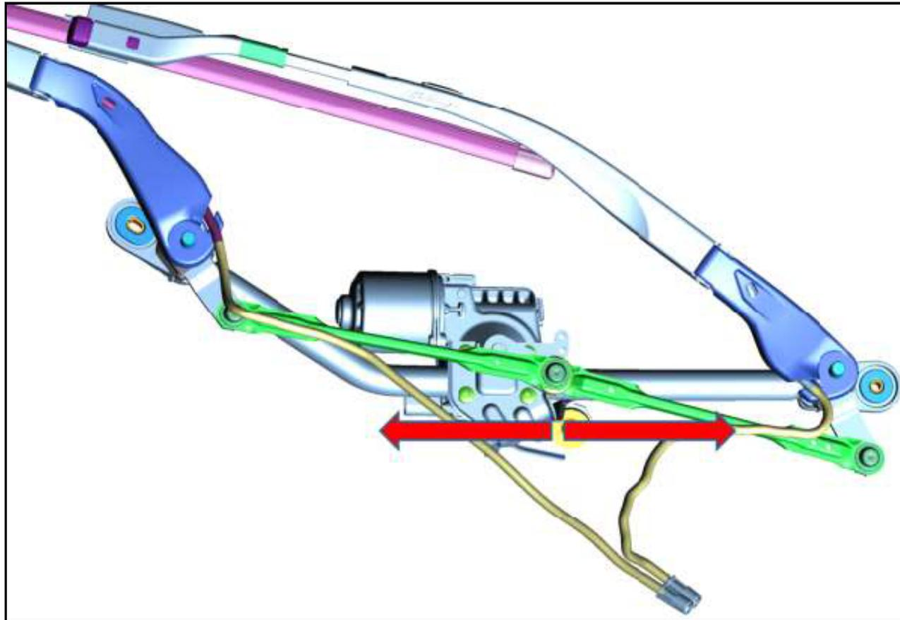
The feature of the electric motor is that it is controlled by electronics which can reverse the control linkage movement. In traditional windshield wiper mechanisms, the electric motor always turns the same way. The motion of the two blades is obtained by means of a cam present in the control mechanism.
