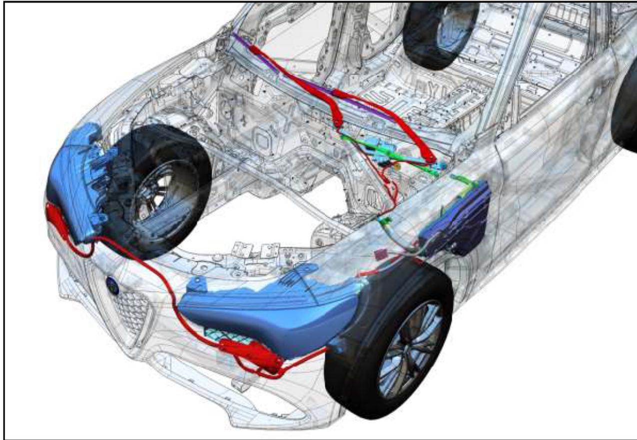
The windshield washer system implements headlight washers only if the vehicle is equipped with top level headlights (Xenon 35W).
