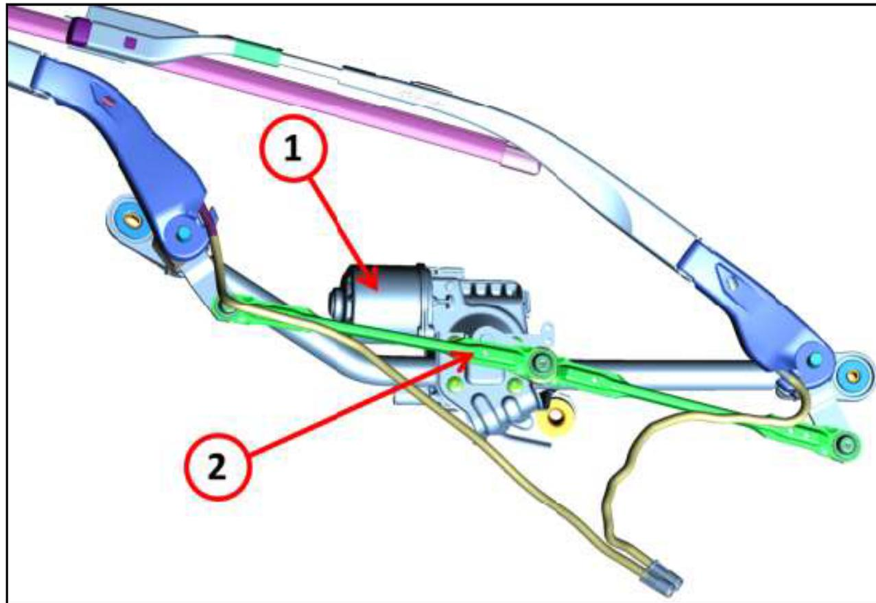
The windshield wiper mechanism consists of a Local Interface Network (LIN) bus controlled electric motor (1) which operates the control linkage (2) of the two arms, to which the rest of the wiper linkage and wiper blades are connected.
