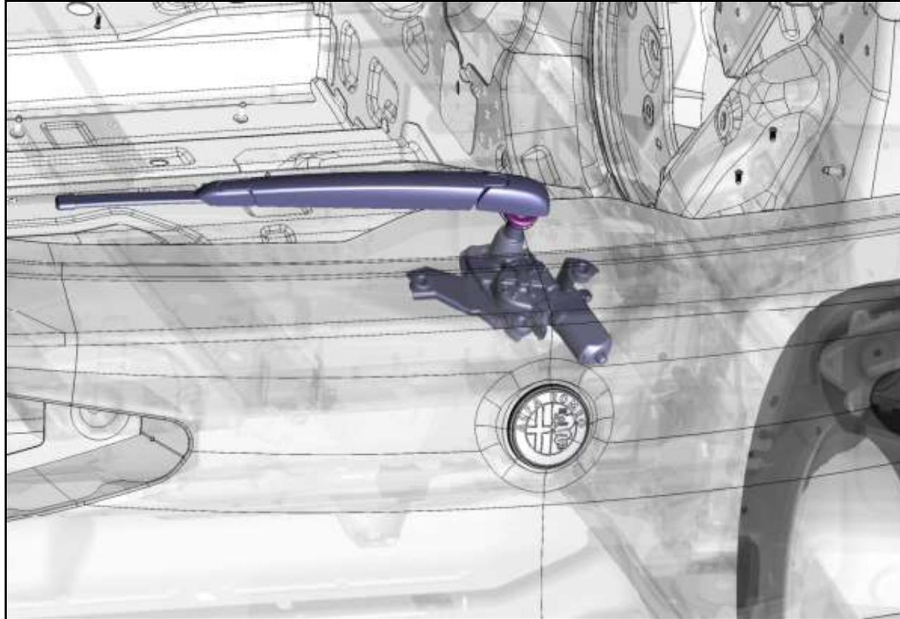
The rear window wiper mechanism consists of an electric motor which operates a cam for controlling the arm to the ends of which the wiper blades are coupled.
