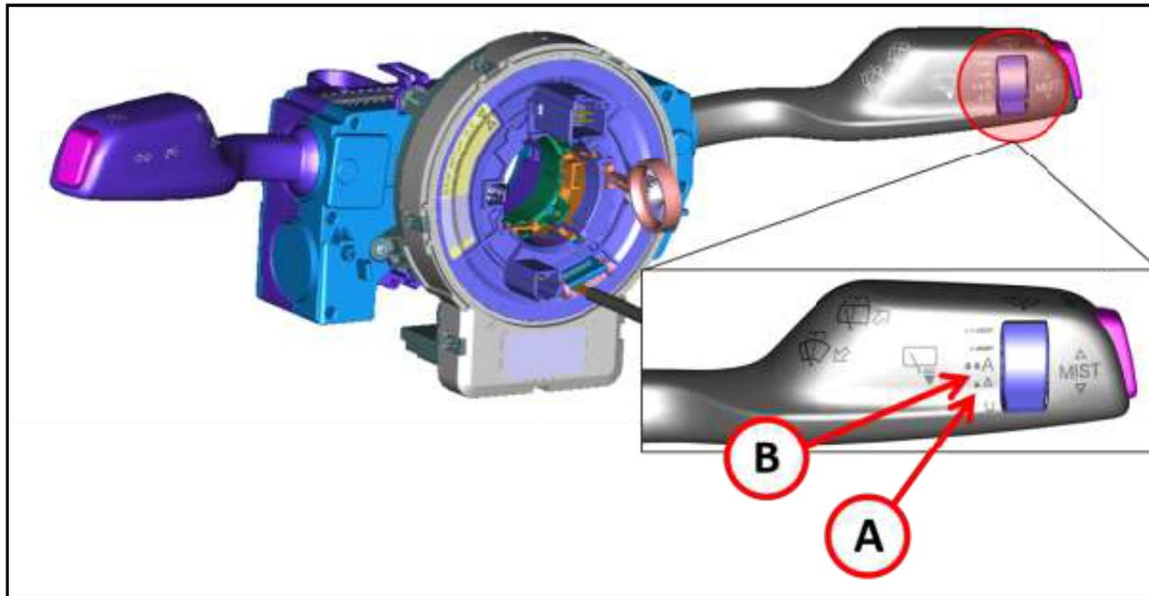
Automatic activation can be selected by the user by setting the windshield wiper control position to one of the two initial positions. The user can set the rain sensitivity level of the automatic function by selecting position A or B.
